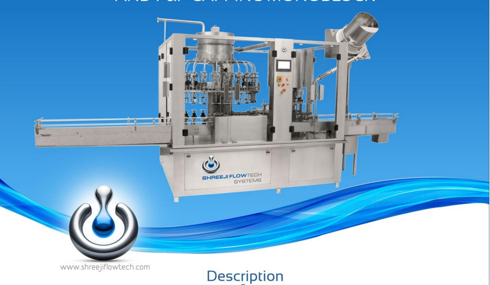
Gear Pump Filling and capper mono block offers flexibility for wide range of liquids with ease of simply. Gear pump fillers are positive displacement pumps with self-priming features. Pumps can fill minimum to maximum fill volume without any mechanical setting by HMI such as a flow meter. Gear Pump filling is a cheaper option of flow meter filling.
